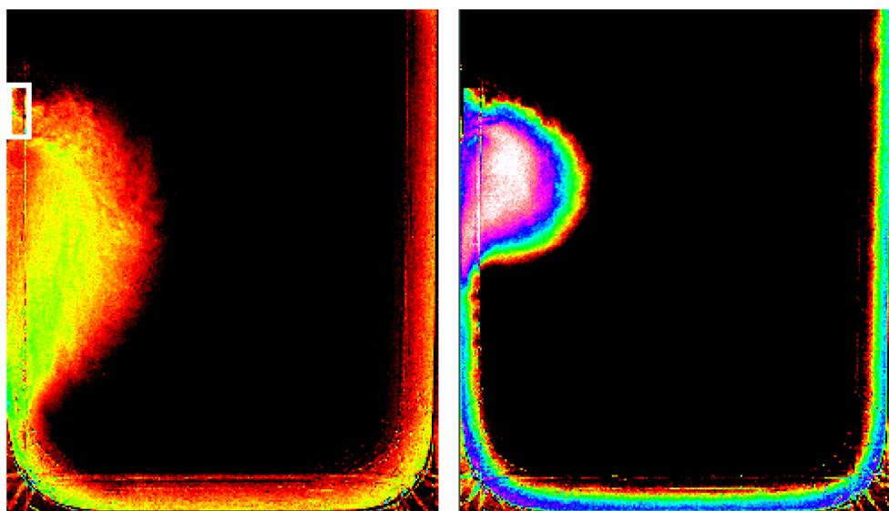
Figure 2: Plan view of typical experiments. The two main features of the outflow vortex and boundary current can clearly be seen in both images.
