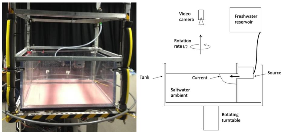
Figure 1: Experimental setup – photograph of tank and schematic diagram.
