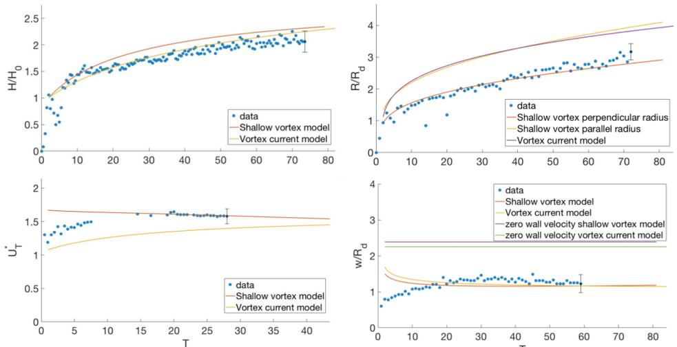
Figure 3: Comparison of the experimental data with the new time-dependent model for the vortex depth  $H$ , radius  $R$ , and current velocity  $U_T$ , width  $w$ .
